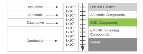
**Note**: Electrical resistivity measurement in accordance with ABC3D standard method based on standard injection molded IZOD specimens, processed according to parameters provided before (General Processing Guidelines for Injection Molding).
